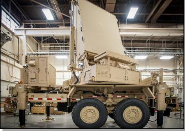
Mounted on its 5-ton FMTV prime mover, the Q-53 can be rapidly deployed and integrated into the tactical battlefield with heavy, medium and light forces. The Target Acquisition Subsystem contains the radar on a singleprime mover and tows the power generator. This package performs all missions of the Q-53 for shorter durations.
